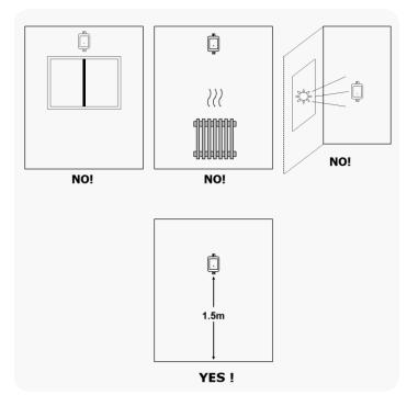
Picture 3 - Device positioning
