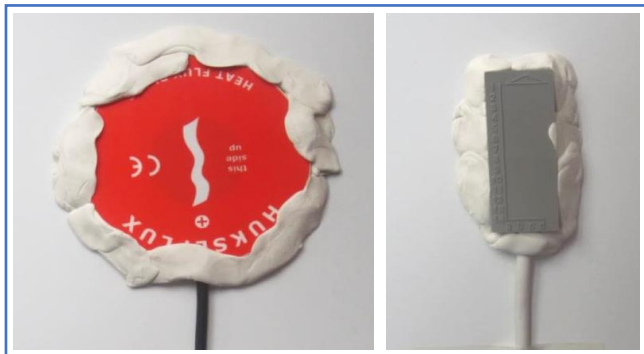
Picture 6 - Thermo-fluxmeter plate and temperature transducer fixing with adhesive rubber or paper ribbon
