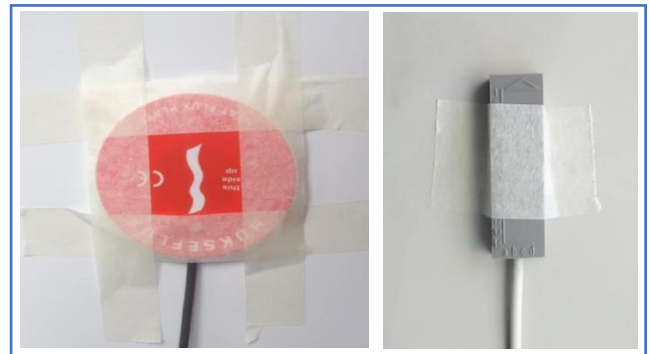
Picture 6 - Thermo-fluxmeter plate and temperature transducer fixing with adhesive rubber or paper ribbon
