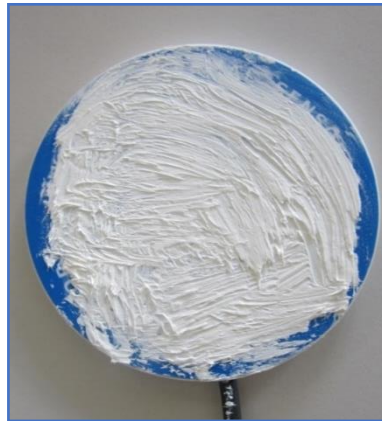
Picture 5 - Thermo-fluxmeter plate and temperature transducer with thermo-conductive paste
